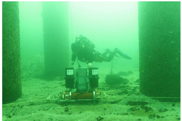
This prototype of an underwater fuel cell system was tested for 8 weeks in the Baltic Sea near the German coast in order to demonstrate the working principle as a first step. For this purpose a small system was selected with low output power and small fuel and oxidant amounts. At the moment there are some further improvements in development like more cells, the extension of the electrode surface and other fuels.
